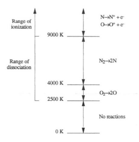
Figure 1. Temperature ranges for air dissociation and ionization (for air at approximately 1 atm).
